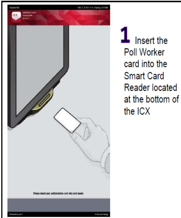
**1** Insert the Poll Worker card into the Smart Card Reader located at the bottom of the ICX
