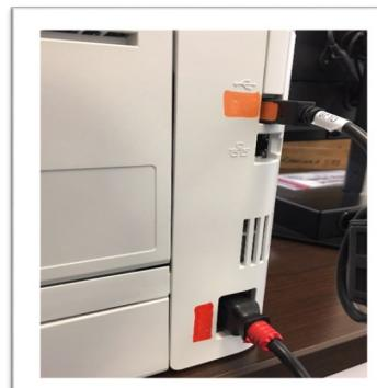
9. Take other end of the **red** printer power cord and plug into the black power strip on the back of the blue cart.
